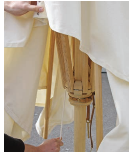
3. Press the tensioning struts lightly outward and pull on the Perlon rope (low tension).
