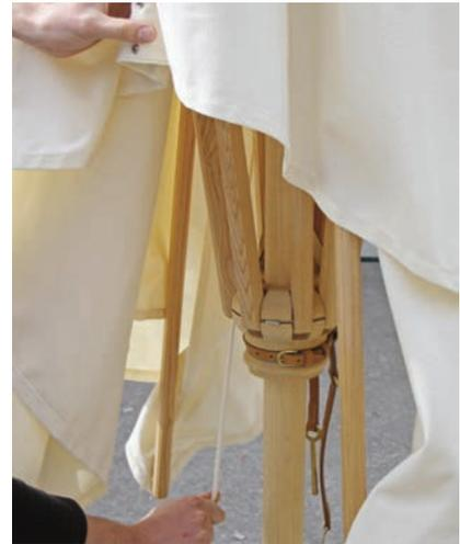
3. Press the tensioning struts lightly outward and pull on the parasol rope (low tension).
